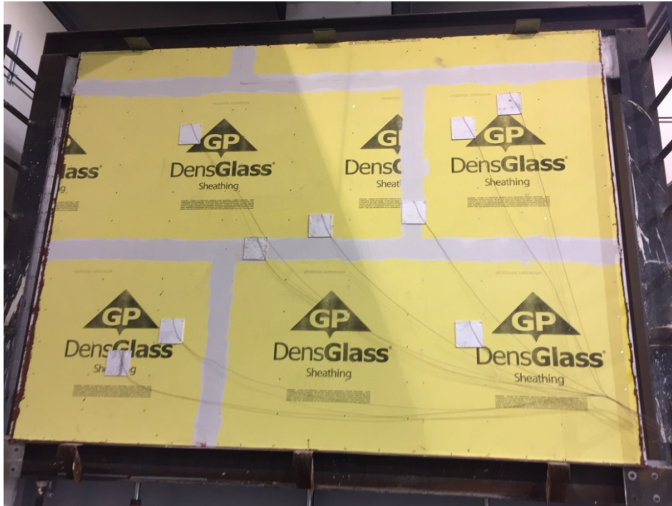
Figure 7: The unexposed face prior to the fire test.
