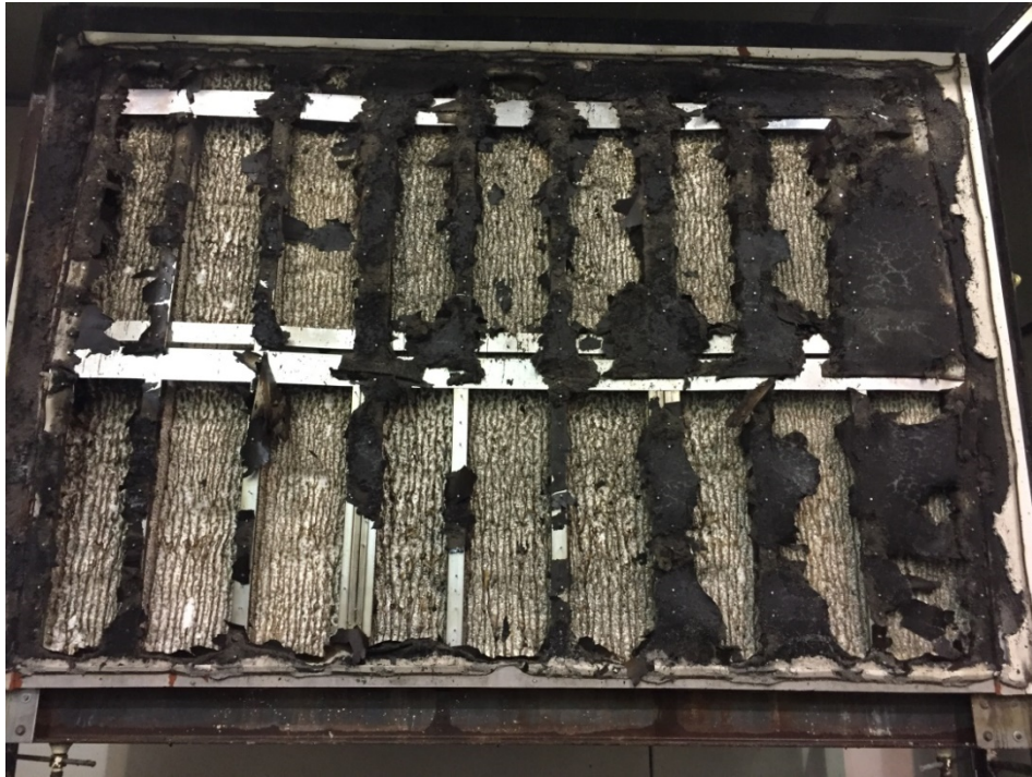
Figure 11: The exposed face after the hose stream test.
