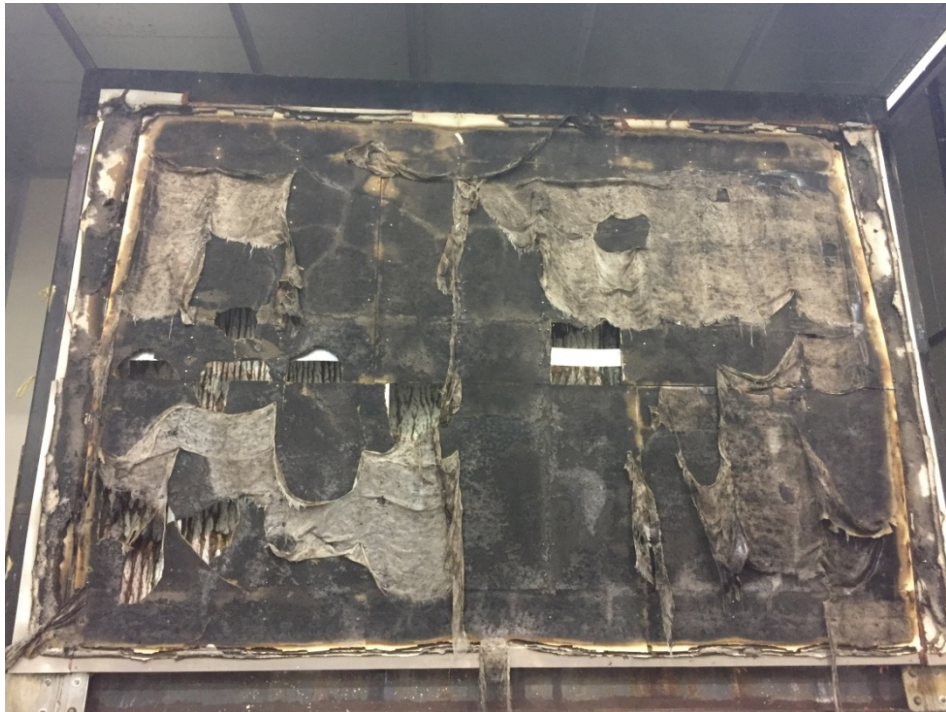
Figure 8: The exposed face after the hose stream test.
