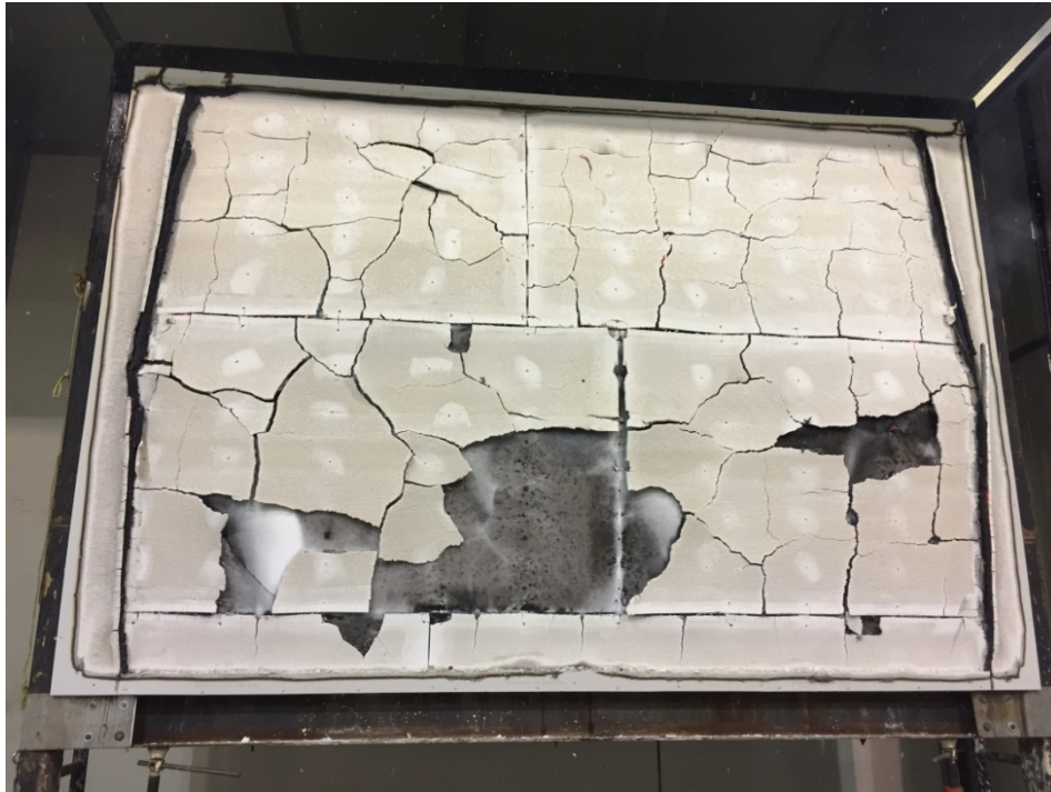
Figure 7: The exposed face after the fire test.
