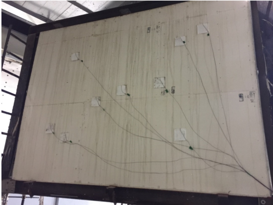
Figure 9: The unexposed face after the hose stream test.
